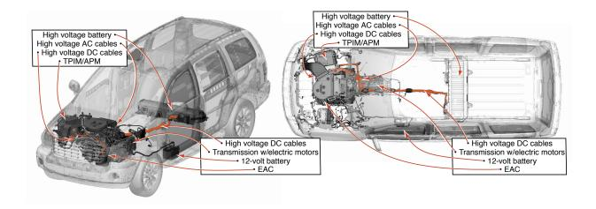
Safety Features – In most accident situations an automatic shut-off of the high voltage system is triggered and the flow of energy from the high voltage system is disabled.
