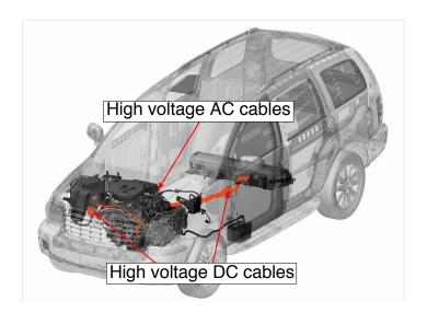
Note that there are also AC high voltage cables and DC high voltage cables located in the engine compartment. The AC cables travel from the TPIM to the transmission. The DC cables travel from the TPIM to the EAC. Both the AC and the DC cables located in the engine compartment are orange in color.
