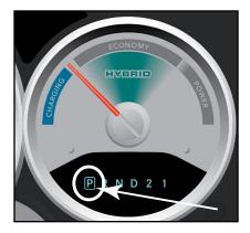
The park pawl will normally engage when the PARK position is selected and the vehicle speed is less than about 3 mph (4.8 km/h). After the park pawl is engaged, vehicle travel due to rolling is limited to no more than 6 in (150 mm). Chock the wheels to prevent any undesired vehicle travel.
