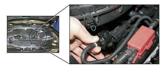
Disconnecting the 12-volt battery negative cable also disables the supplemental restraint system (SRS). The SRS may remain powered for up to two minutes after the vehicle is disabled.
