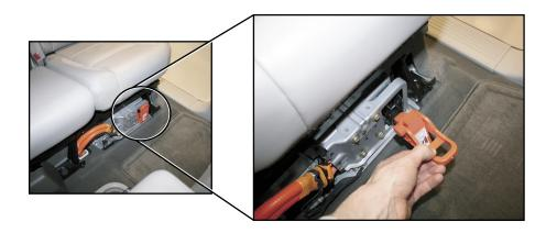
The service disconnect is located on the driver side front of the high voltage battery module. The plastic disconnect is colored bright orange. By removing this disconnect the high voltage battery circuit is interrupted.
