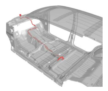
From the high voltage battery the DC cables are routed toward the middle of the vehicle, down through the floor pan, and then forward, on the underside of the vehicle, between the transmission and the floor, until just before the engine compartment. From there, the DC cables are routed towards the passenger-side of the vehicle and up to the TPIM.
