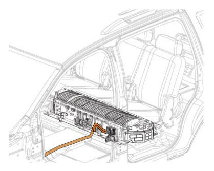
The DC high voltage cables originate at the high voltage battery. The connection is located on the driver side of the vehicle on the front of the battery.
